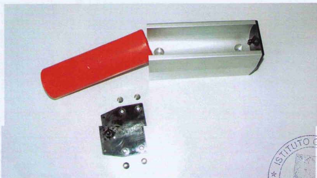
After-test photos of the dismantled roller buffers
