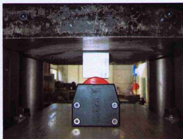
Photos of roller buffers during testing
